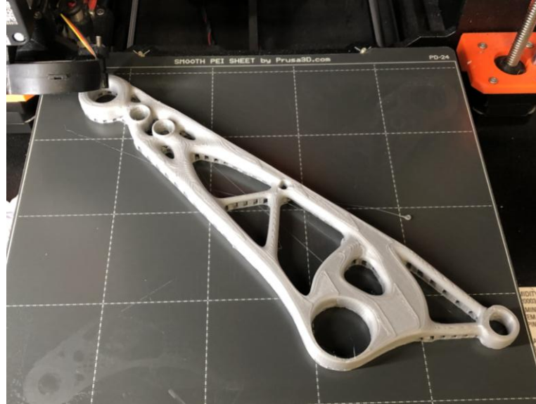
Figure 1 3D printer producing the optimized prototype, own source.
