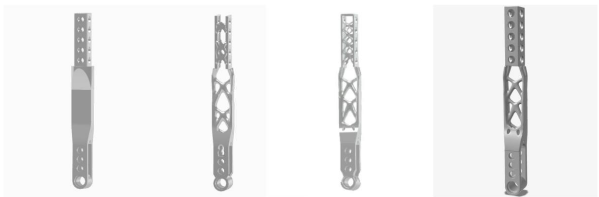
Figura 9: Optimization through Generative Design and Refinement.
