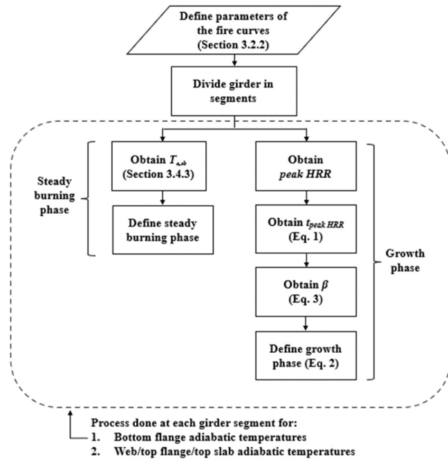
Fig. 3. Flowchart summarizing the process of definition of the parametric fire curves.
