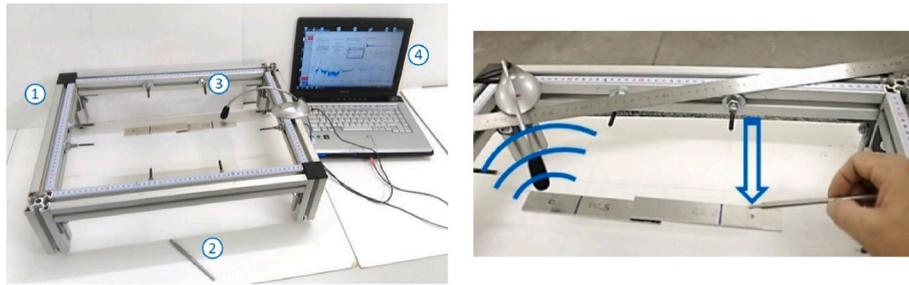
Fig. 2. Sound pressure level measurement system. (1) Universal wire support (2) Impact rod (3) USB microphone (4) Laptop with dedicated software.
