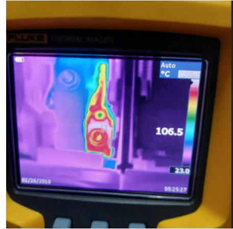
(b) Thermal imaging of the hot spot event
