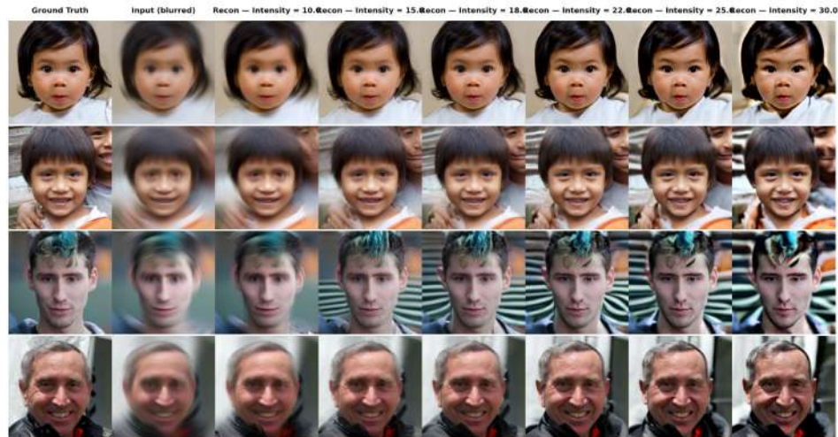
Figure 23: DPS reconstruction results across a range of guidance intensities for an input corrupted by Rotation blur (intensity 20.0).
