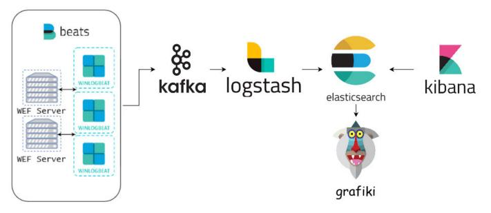
Figure 2. Event Based Detection System (EBDS) Diagram.
