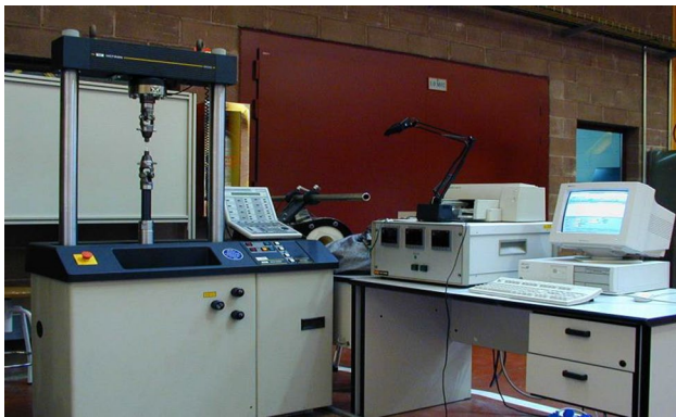
Fig. 6. Instron universal testing machine, model 8516 with a maximum load of 100 KN used to perform either tensile tests or compressive tests
