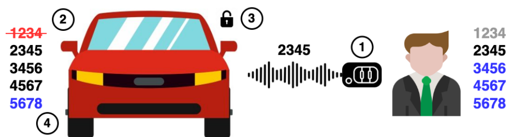
Figure 1. Operation of rolling codes.
