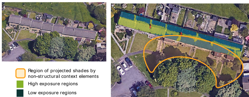
Fig. 7. Example of occlusions produced by non-structural surrounding elements of higher dimension.
