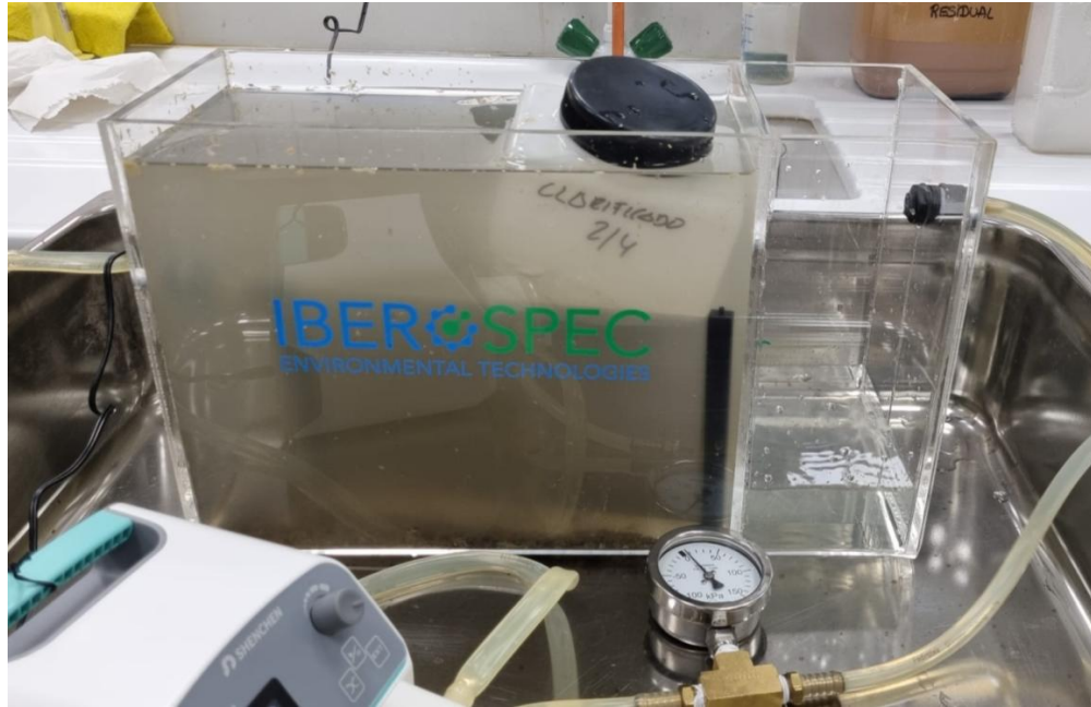
Figure 2 - Filtration process of clarified sample, May 21, 2025 (Own elaboration).
