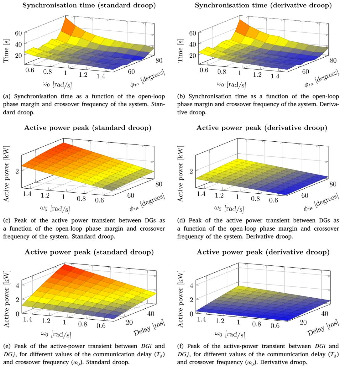
Fig. 4. Fundamental study of the powerflow between two DGs.
