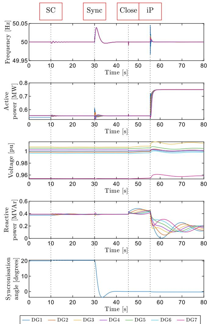
Fig. 11. Simulation results of the synchronisation of the IEEE 69 bus test system to an infinite grid with the proposed control.
