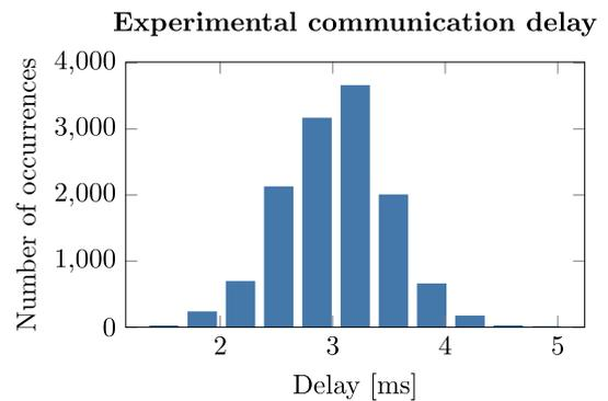
Fig. 8. Histogram of the experimental measures of the communication delay between *DG1* and *DG2* in the laboratory.
