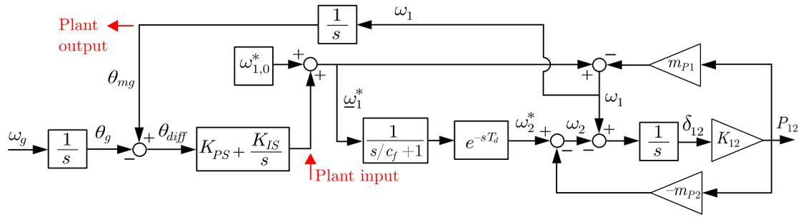
Fig. 3. Block diagram representing the dynamic model of the agent-based secondary controller applied in this work.
