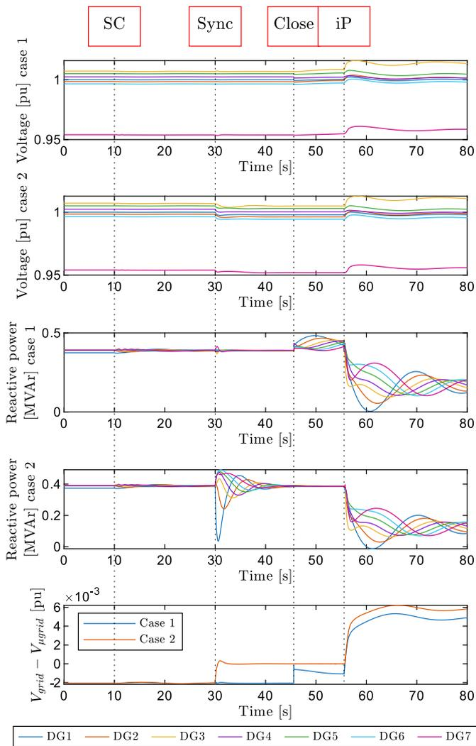
Fig. 12. Voltage, reactive power and voltage amplitude difference ( $V_{grid} - V_{microgrid}$ ) comparison between case 1 (no amplitude difference control) and 2 (amplitude difference control).
