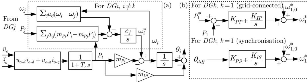
Fig. 2. Primary and secondary controller of a DG. In (a), for any DG except the leader ( $k$ ). In (b), for the leader ( $k = 1$  in this work).
