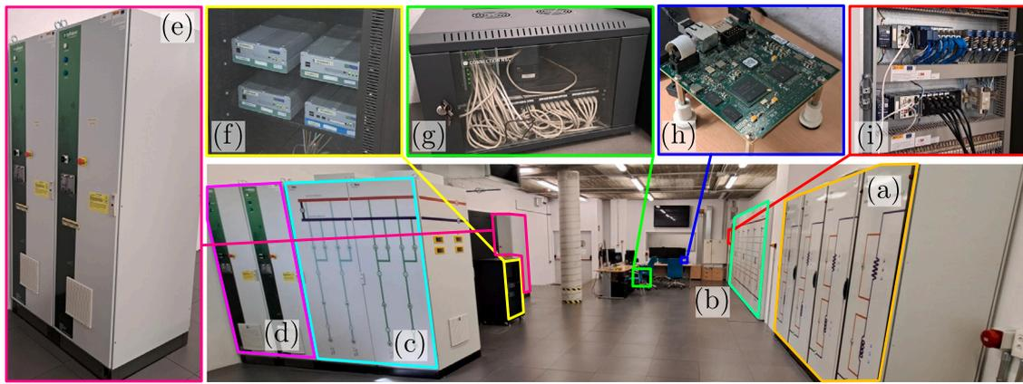
Fig. 7. Pictures of the elements of the laboratory. (a) Line impedances, (b) AC busbars, (c) DC busbars, (d) 75 kVA VSCs, (e) 15 kVA VSCs, (f) real-time computers, (g) communication network switch, (h) single-board RIO and (i) two compactRIO.
