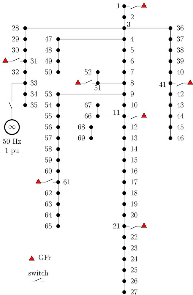
Fig. 10. Single-line diagram of the modified version of the IEEE 69 bus test system.
