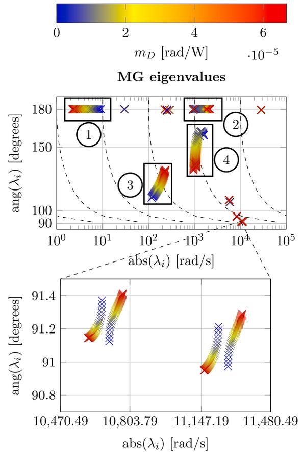
**Fig. 6.** Angle versus absolute value of the MG eigenvalues, for different values of  $m_D$  (see the text for explanations).
