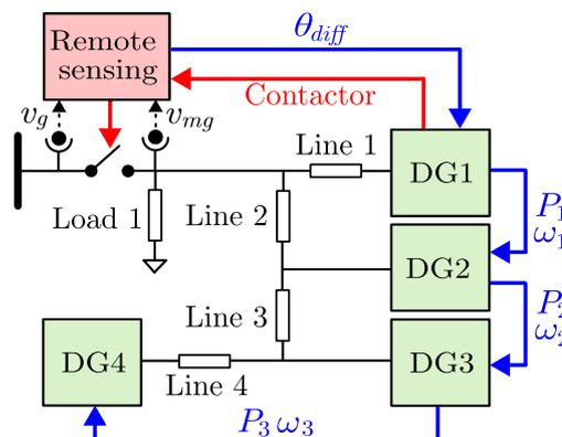
**Fig. 1.** Electrical and control system diagram of the MG studied in this work. Four DGs with a decentralised secondary controller.
