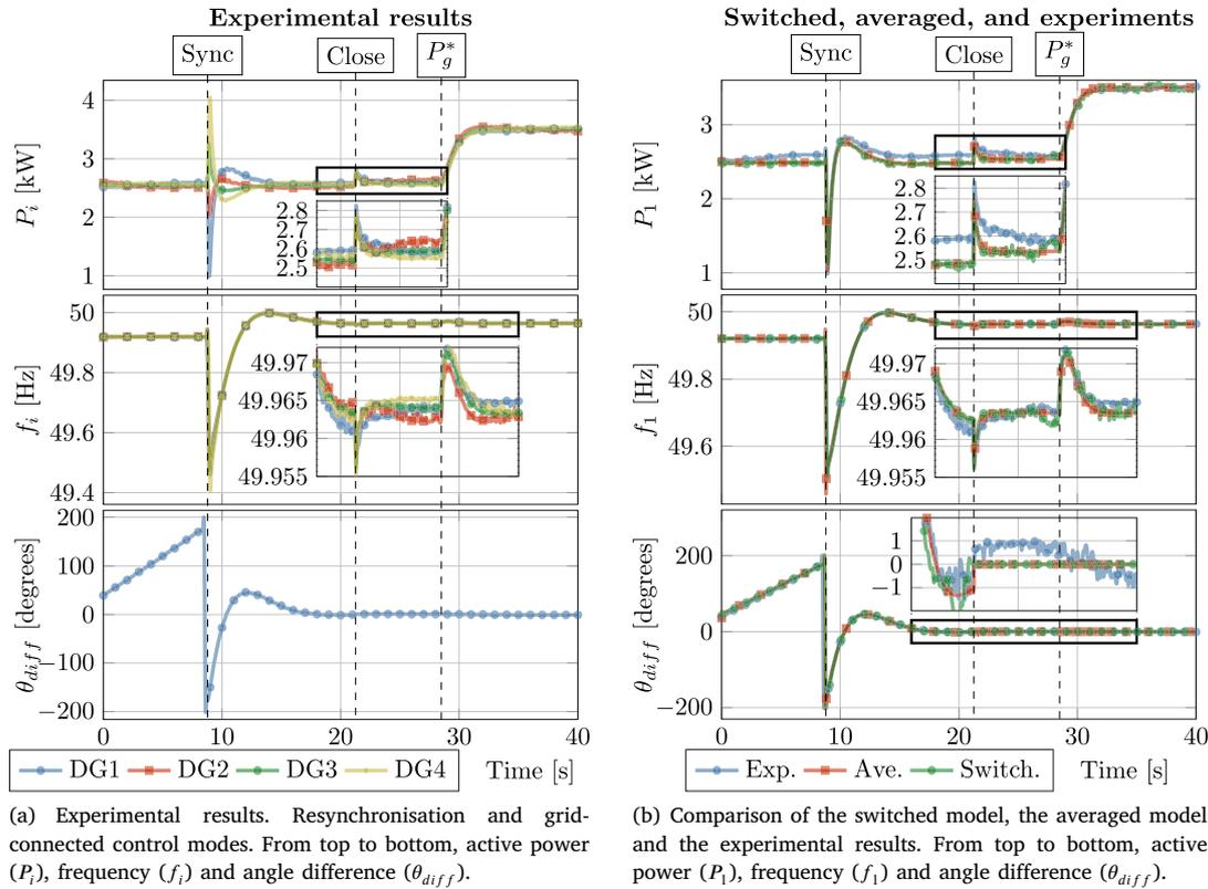
Fig. 9. Comparison of the switched model, the averaged model and the experimental results.
