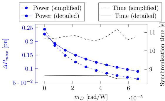
Fig. 5. (blue) Active power peak needed for synchronisation and (black) synchronisation time, for different values of  $m_D$  (dashed) Simplified and (solid) detailed MG model.
