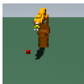
Figure 3. Sample of the BM environment at the episode's beginning. This 64 \times 64 pixel RGB image is the model input. The initial joints and target positions are sampled from two uniform distributions.
