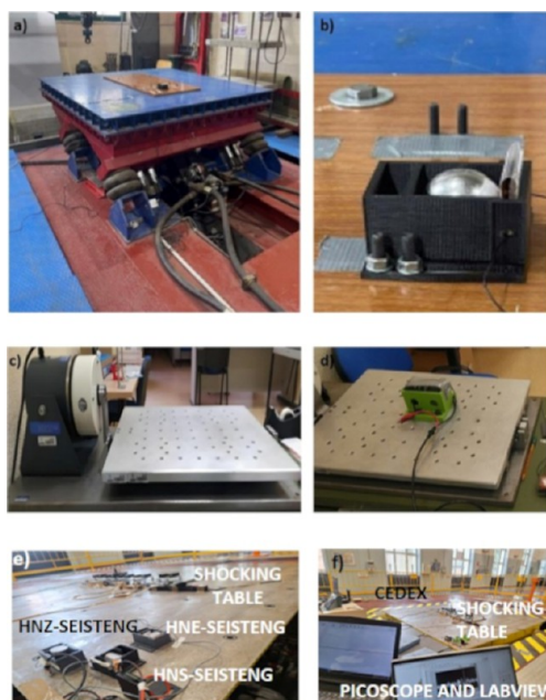
Figure 1. (a) A vibration table from Matest, model C278, on which (b) the TENG case with the TENG inside and the inertial mass is shown; (c) V20 shaker powered with a PA100 amplifier on which (d) the TENG is screwed; (e) different parts of 3D-SEISTENG fixed to the shocking table; and (f) software and setup employed in monitoring the different seismic waves.
