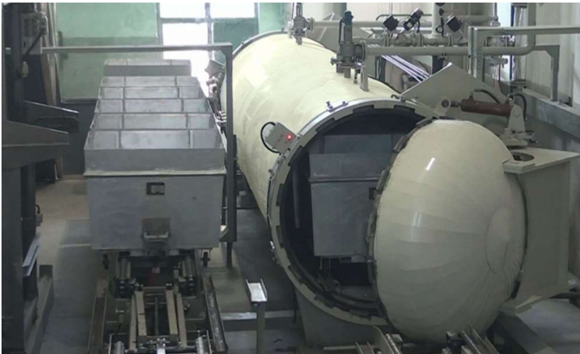
Figure 5: Large-Scale Autoclave for Central Treatment Plants. Source: (Gient)
