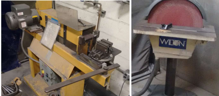
Figures 29 and 30: Rusch machine & design abrasive belt tube and Pipe Notcher, and Wilton Disc Sander
