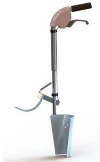
3D design of the shoehorn made with SolidWorks [Claudia Ríos]
