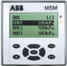
MSM: LC display in the local control cubicle
