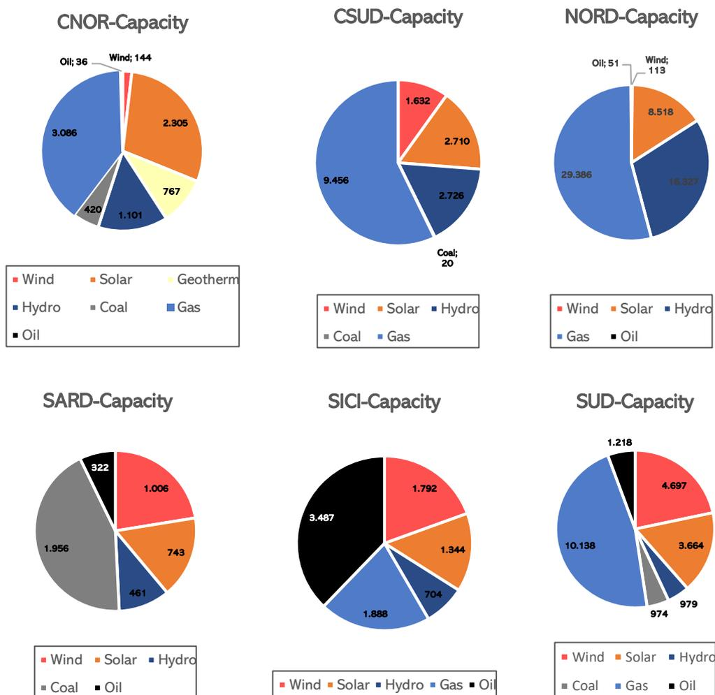
Figure 7: Capacity mix (MW). Reference: own elaboration. Data source: Terna.
