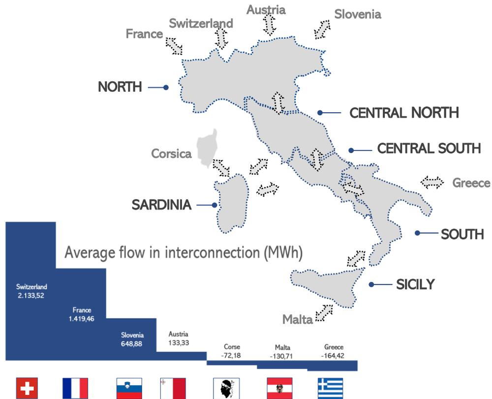
Figure 8: Average flow in interconnection and interconnection diagram. Reference: own elaboration. Data source: Terna.
