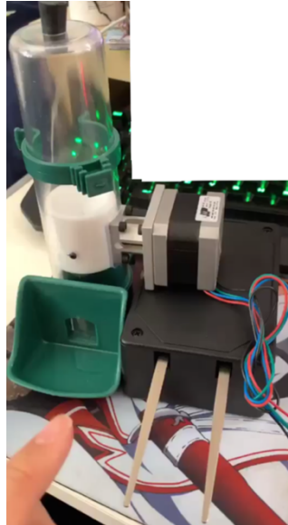
Figure 8: Food dispenser and switches.
