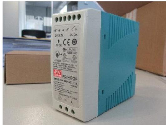
Figure 18. Din rail power supply
