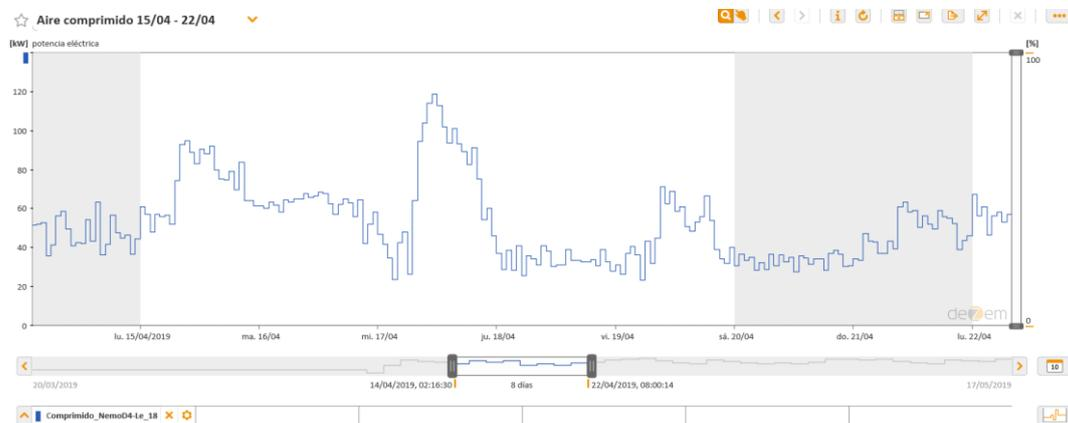
Figure 59. Aire comprimido consumption 15/04 - 22/04
