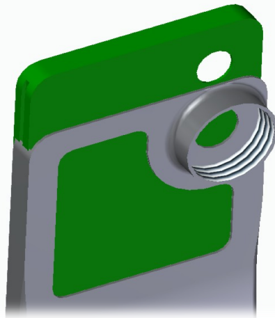
Figura I.8 Housing sliding along the base plate rails. Source: Own preparation. Year 2019.
