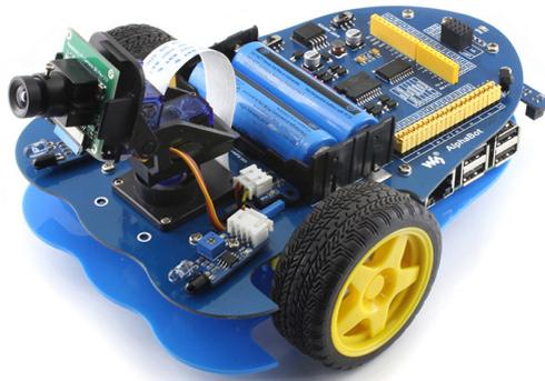
Fig 3 – The AlphaBot robot
