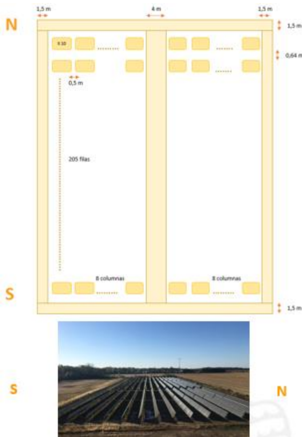
Figure 12. Scheme of the panels' distribution. Source: Own Elaboration.
