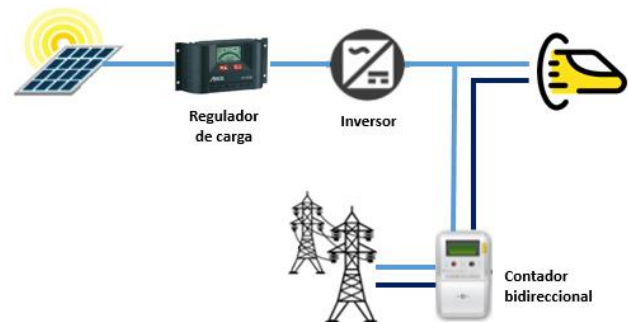
Figure 11. Scheme of the self-consumption mode installation. Source: Own Elaboration.
