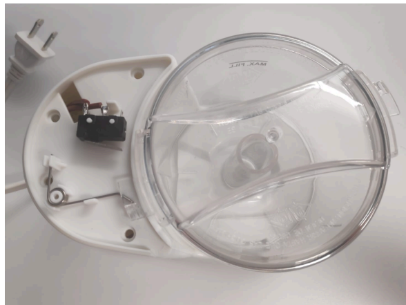
Figure 4. Switch and how it is activated.
