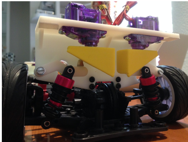
Figure 2. Placed frontal active damping mechanic system.
