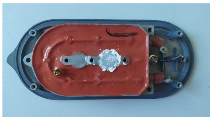
*Figure 8: Ceramic soleplate (grey) and iron plate (garnet)*
