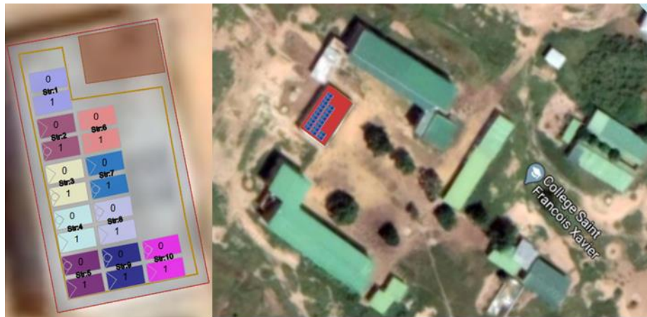
Figure 5: Plan view and distribution of photovoltaic panels.
