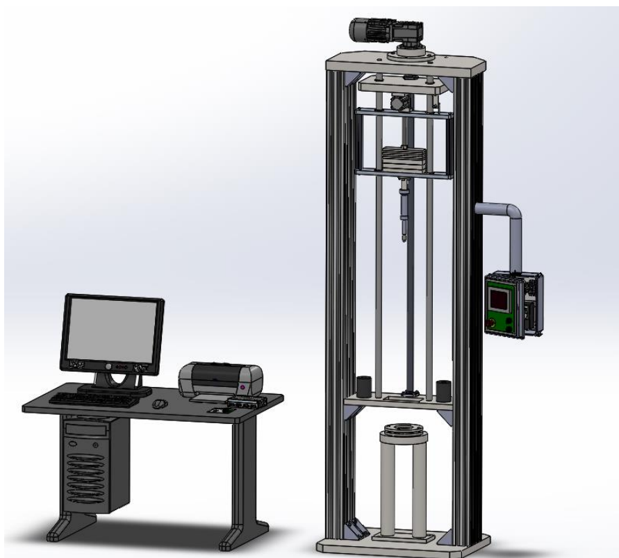
Ilustración 13: Arrangement of equipment for impact testing of polymers and composite materials
