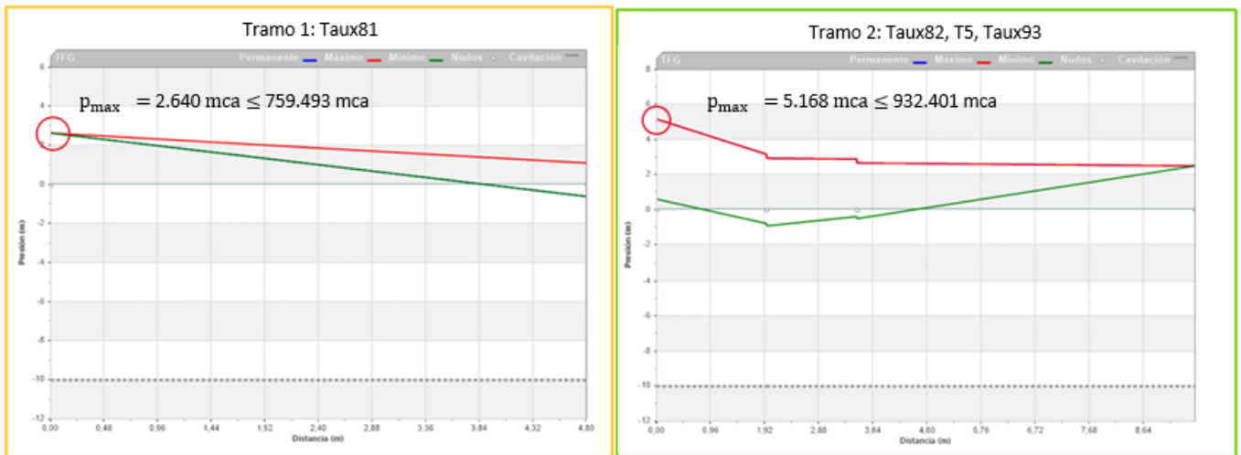
Figura 41. Transient regime: Overpressures, circuit 3, Kaplan turbine with Weise pump
