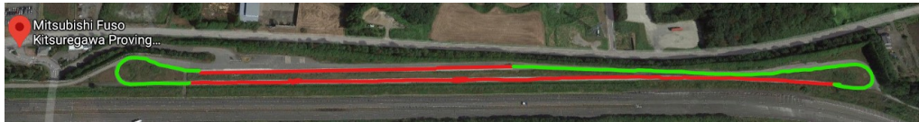
Figure 1.2: Road type distribution along the circuit. Red lines shows the Rough Road part of the circuit and the Green lines the Smooth Road.
