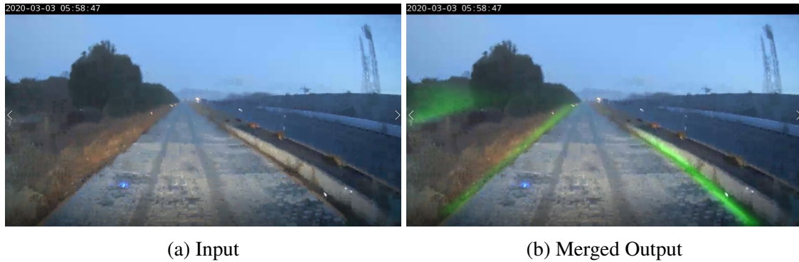
Figure 20: ERFNet_TuSimple Model Output for Smooth Road
