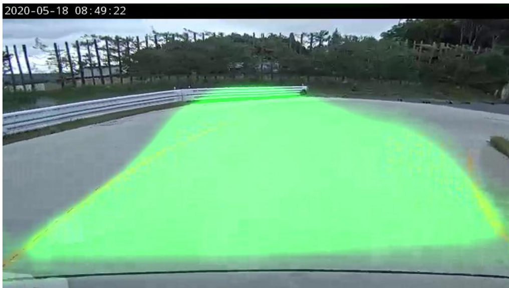
Figure 4.39: ERFNet False positive output prediction 2. It is possible to appreciate the model detects the road fence as part of the road.
