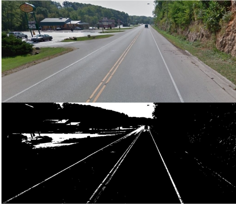
Figure 2.1: Example of the Canny Edge Detection model of an image of a road.
