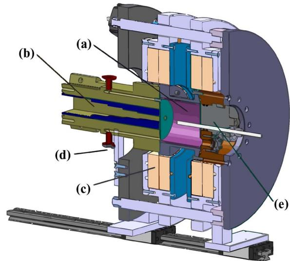
Fig. 1. View of plasma chamber and main subsystems. (a) Plasma chamber. (b) MW impedance adaptor. (c) Coil pancakes. (d) Pressure gauge inlet. (e) Diagnostic port.
