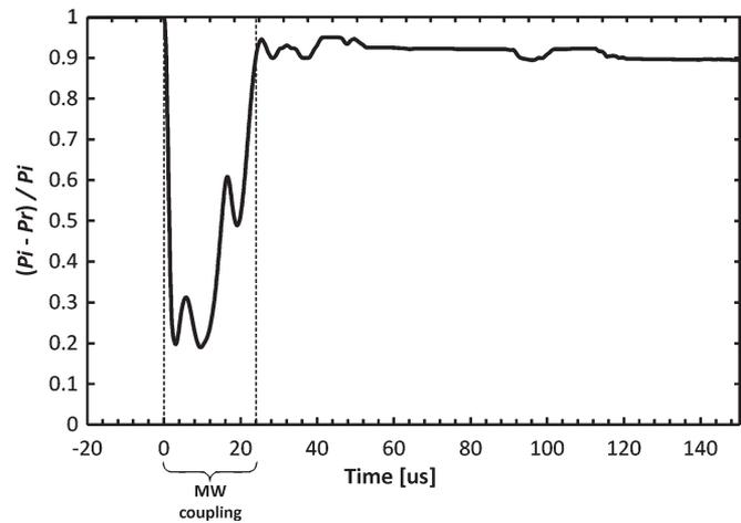
Fig. 6. Typical relative absorbed power  $(P_i - P_r)/P_i$  calculated from direct measurements showing the MW-coupling time definition as proposed.
