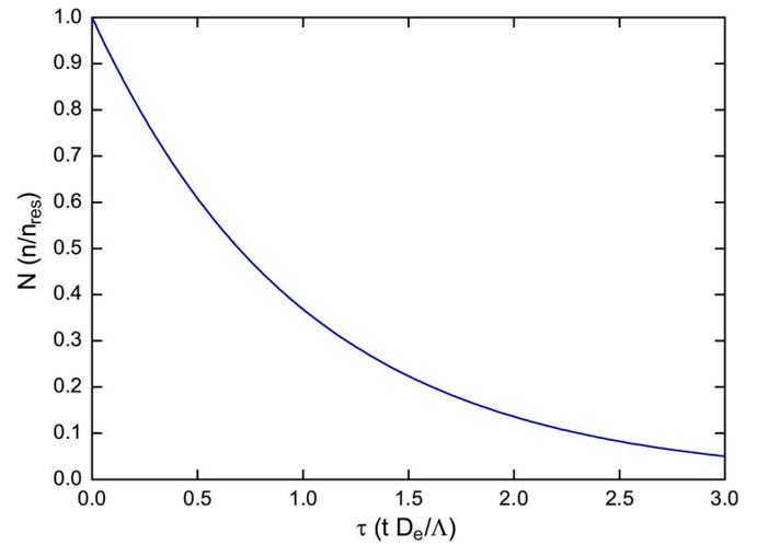
Fig. 14. Calculation of seed electron density temporal evolution at  $r = 0$ .
