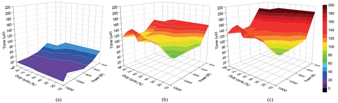
Fig. 8. Breakdown times for a flat  $B_z < \text{ECR}$  magnetic field distribution corresponding to Figs. 2(a) and 3(a) for a hydrogen pressure of  $6.2 \times 10^{-3}$  mbar. (a) MW coupling time. (b) Plasma formation time. (c) Total breakdown time as the sum of the previous values.
