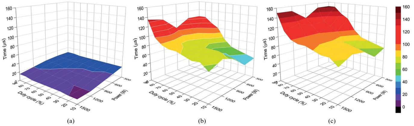
Fig. 10. Breakdown times for a flat  $B_z \simeq$  ECR magnetic field distribution corresponding to Figs. 2(b) and 3(b) for a hydrogen pressure of  $6.2 \times 10^{-3}$  mbar. (a) MW coupling time. (b) Plasma formation time. (c) Total breakdown time as the sum of previous values.
