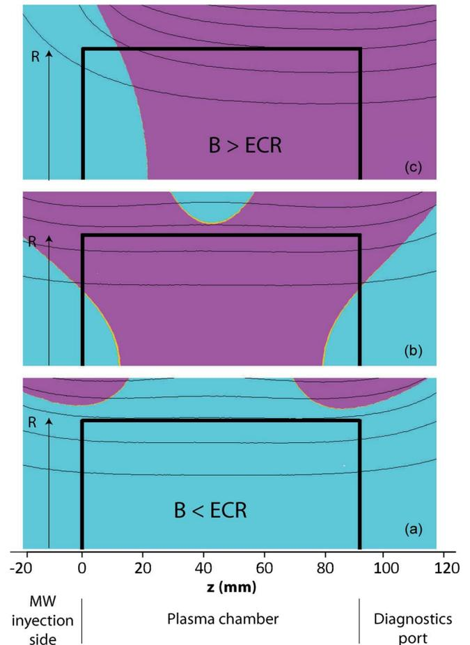
Fig. 3. Two-dimensional representation of magnetic profiles used during experiments showing the volumes for (violet)  $B > \text{ECR}$  and (blue)  $B < \text{ECR}$ , where the border between both volumes is the  $B \simeq \text{ECR}$  surface for each case: (a) Symmetric  $B_z < \text{ECR}$  magnetic profile; (b) Symmetric  $B_z \simeq \text{ECR}$  profile; (c) Asymmetric  $B_z > \text{ECR}$  magnetic profile. Symmetric half plasma chamber profile is represented by a full black line.
