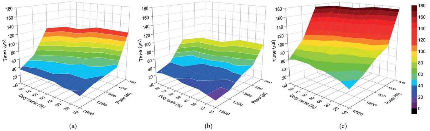
Fig. 11. Breakdown times for a flat  $B_z >$  ECR magnetic field distribution corresponding to Figs. 2(c) and 3(c) for a hydrogen pressure of  $3.8 \times 10^{-3}$  mbar. (a) MW coupling time. (b) Plasma formation time. (c) Total breakdown time as the sum of the previous values.
