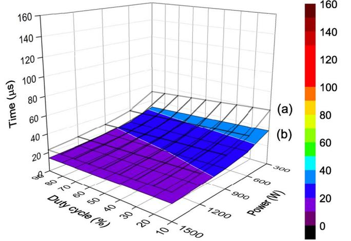
Fig. 15. Calculation of breakdown times for (a)  $3.8 \times 10^{-3}$  mbar and (b)  $6.2 \times 10^{-3}$  mbar.
