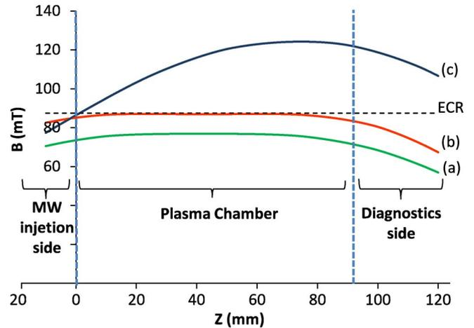
Fig. 2.  $Z$ -axis magnetic profiles used during experiments. (a) Symmetric  $B_z < \text{ECR}$  magnetic profile. (b) Symmetric  $B_z \simeq \text{ECR}$  profile. (c) Asymmetric  $B_z > \text{ECR}$  magnetic profile.
