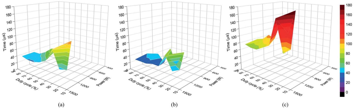
Fig. 7. Breakdown times for  $B_z < \text{ECR}$  magnetic field distribution corresponding to Figs. 2(a) and 3(a) for a hydrogen pressure of  $3.8 \times 10^{-3}$  mbar. (a) MW coupling time. (b) Plasma formation time. (c) Total breakdown time as the sum of the previous values.
