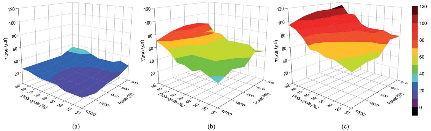
Fig. 12. Breakdown times for a flat  $B_z > \text{ECR}$  magnetic field distribution corresponding to Figs. 2(c) and 3(c) for a hydrogen pressure of  $6.2 \times 10^{-3}$  mbar. (a) MW coupling time. (b) Plasma formation time. (c) Total breakdown time as the sum of previous.
