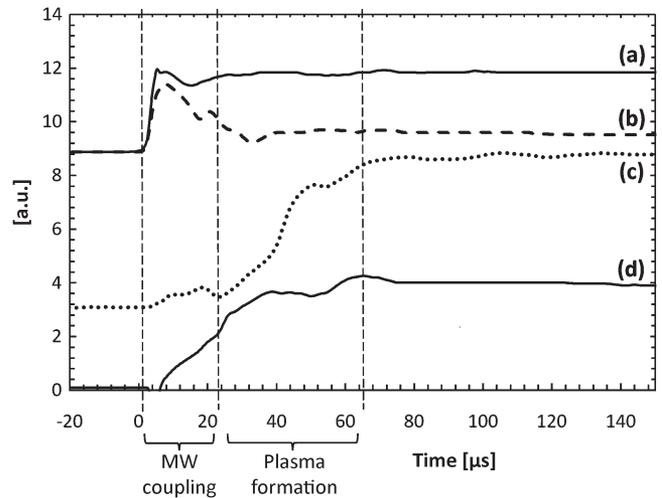
Fig. 5. Typical oscilloscope signal for measuring breakdown times. (a) Incoming power. (b) Reflected power. (c) Plasma emitted light. (d) Probe current.
