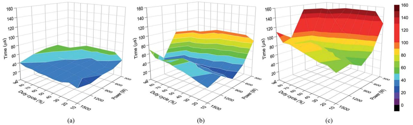
Fig. 9. Breakdown times for a flat  $B_z \approx \text{ECR}$  magnetic field distribution corresponding to Figs. 2(b) and 3(b) for a hydrogen pressure of  $3.8 \times 10^{-3}$  mbar. (a) MW coupling time. (b) Plasma formation time. (c) Total breakdown time as the sum of previous values.
