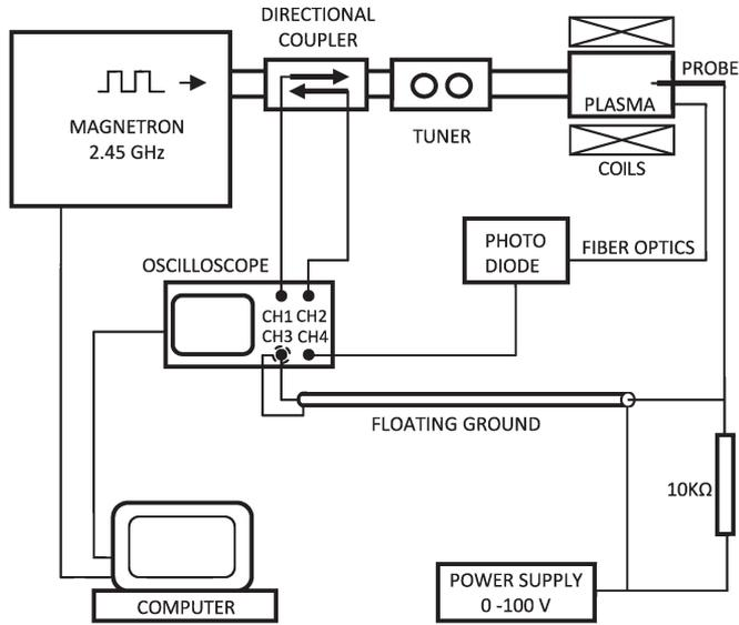
Fig. 4. Experimental setup for breakdown time measurement.
