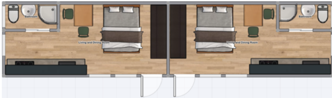
20' CONTAINER DESIGN WITH TWO HOUSES
