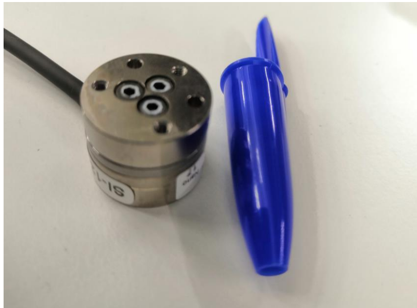
Figure 3. Load cell ATI Nano17 with pen cap for scale.
