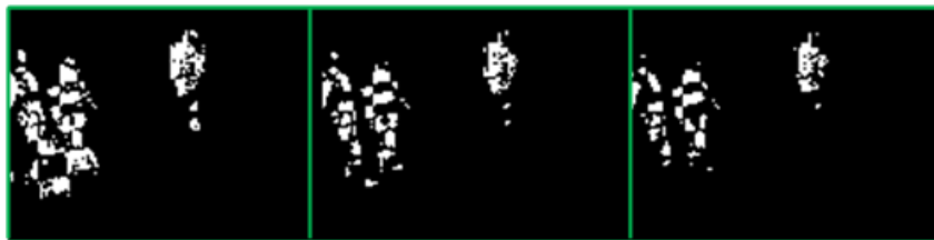
Figure 2.10. Tests for different values of v_{min} on frame 250 in video 1. Left to right: (i) v_{min} = 5 , (ii) v_{min} = 8 and (iii) v_{min} = 10 .
