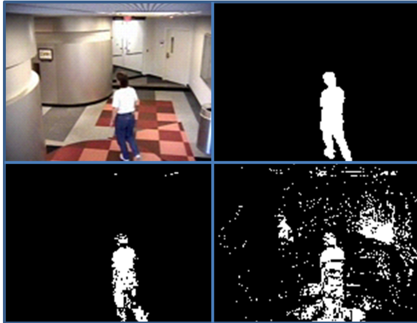
Figure 2.15. Test results on video 3. Upper row: image of video 1 (left) and ideal segmentation (right). Lower row: segmentation obtained with the MGM+RTDENN (left) and the MGM (right) algorithms.
