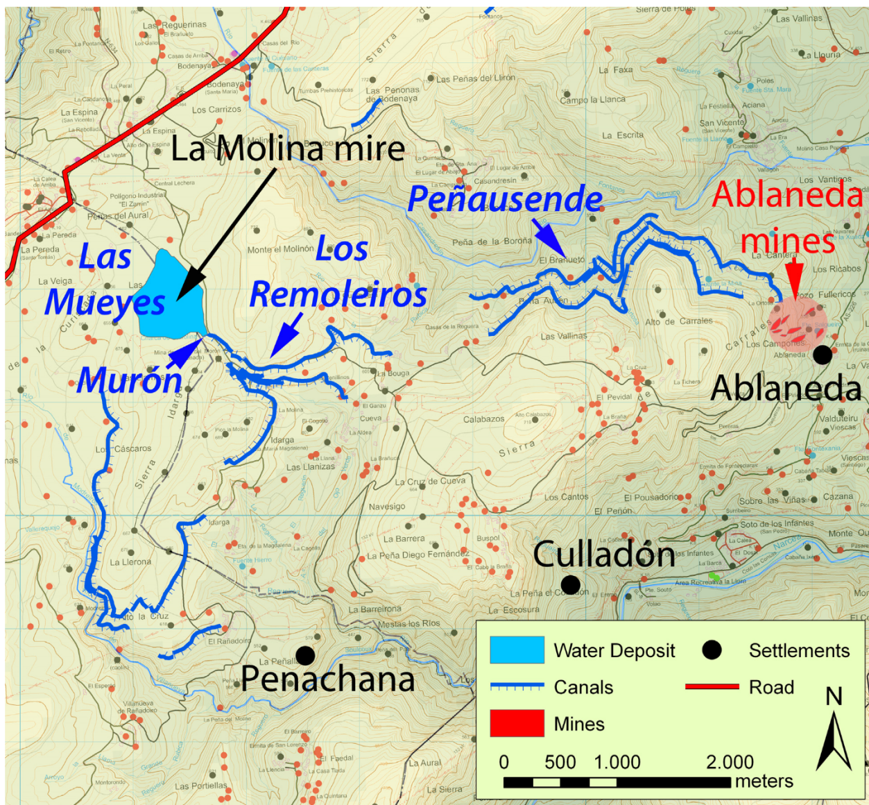
Fig. 2. Mining complex of Ablaneda, including the mines, the canals and the deposit at La Molina ( Las Mueyes ), as interpreted from high-resolution satellite imagery. Associated microtoponyms mentioned in the text are shown in italics. Settlements belong, surely or presumably -given the scarce data available and other regional morphologies-, to the Roman period, when the mine was active. The road is the itinerary of the medieval communication route which could presumably have existed also previously.
