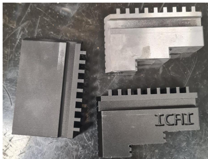
FIGURE 2: ORIGINAL LATHE GRIPPER (TOP RIGHT) AND TWO ADDITIVE PRINTED PROTOTYPES
