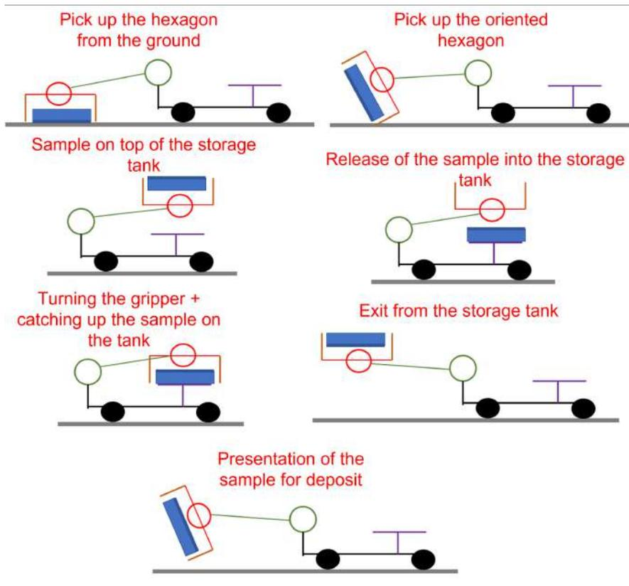
Figure 24: Sample of how the robot works
