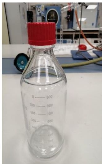
Figure 6. BMP Batch Bottle Resealed with Silicone Paste. Source: Own.
