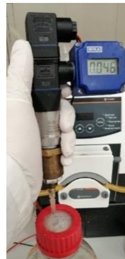
Figure 8: Custom-Built BMP Bottle Barometer. Source: Own.
