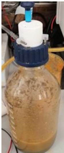
Figure 20: Prepared Semi-Continuous BMP Bottle. Source: Own.
