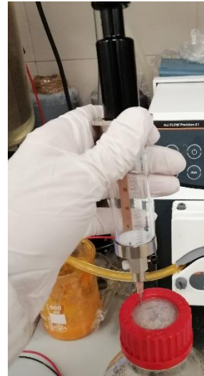
Figure 46: Biogas Sample Collection during Collection from BMP Batch Bottle. Source: Own.
