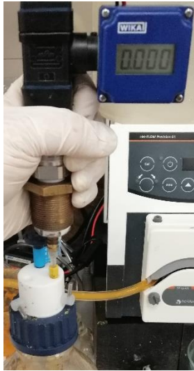
Figure 49: BMP Semi-Continuous Bottle Pressure Measuring. Source: Own.
