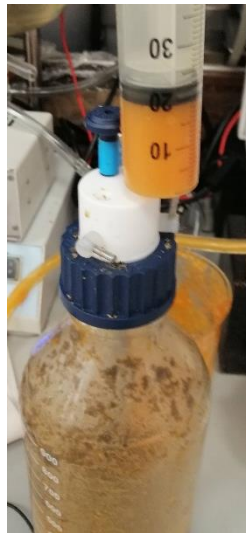
Figure 66: Semi-Continuous Bottle Feed Injection 2. Source: Own.
