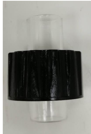
Figure 31: Detailed pH Port Fitting. Side View. Source: Own.
