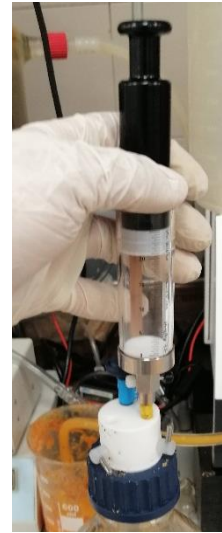
Figure 50: Biogas Sample Collection during Collection from BMP Semi-Continuous Bottle. Source: Own.
