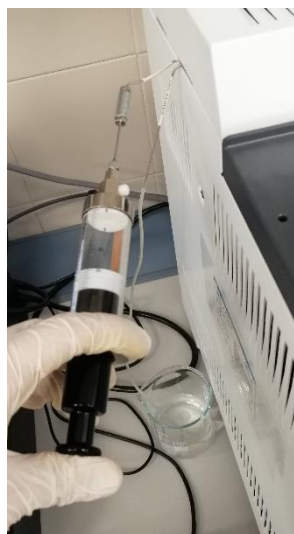
Figure 63: Biogas Sample Injection Representation. Source: Own.
