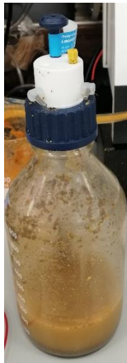
Figure 51: Depressurization of BMP Semi-Continuous Bottle. Source: Own.
