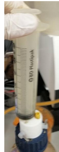
Figure 67: Semi-Continuous Bottle Feed Injection 3. Source: Own.
