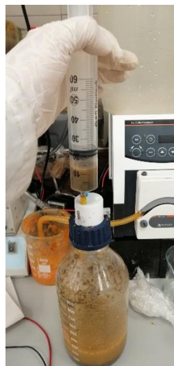
Figure 56: Sludge Extraction from Semi-Continuous Bottle. Source: Own.
