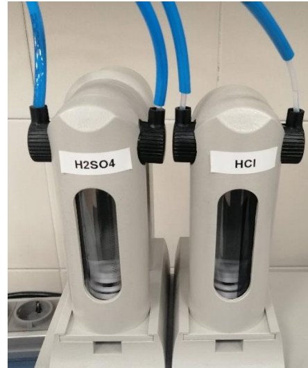
Figure 55: Acid Pumps Used during VFA Testing. Source: Own.
