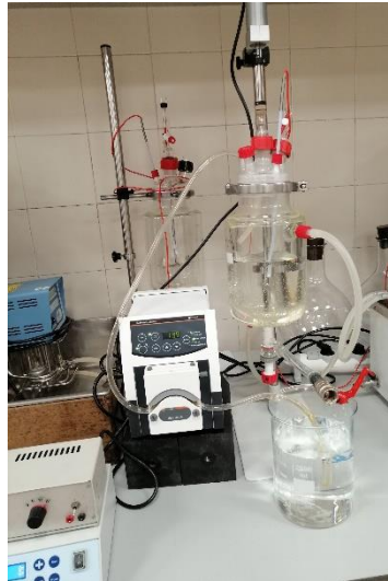
Figure 33: Final Semi-Continuous Reactor Set-Up. Source: Own.
