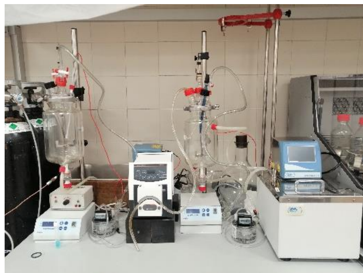
Figure 29: Final Batch Reactor Set-up. Source: Own.
