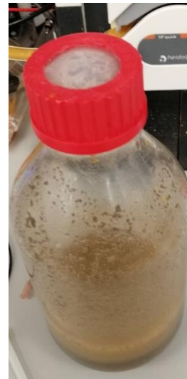
Figure 48: BMP Batch Bottle Resealed with Silicone Paste. Source: Own.
