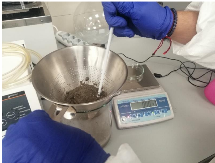
Figure 35: Sludge Filtering to Determine Density. Source: Own.
