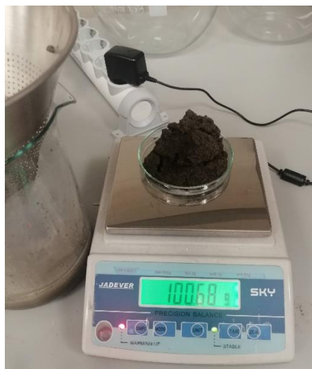
Figure 36: Filtered Sludge Weighing. Source: Own.
