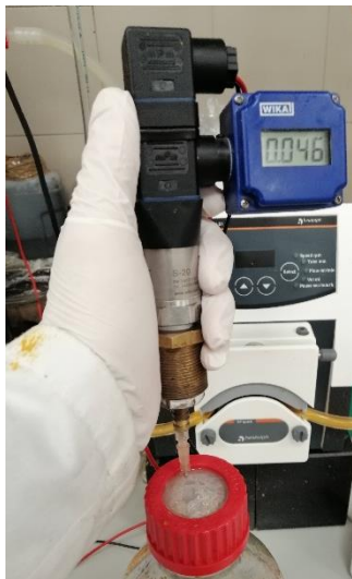
Figure 43: BMP Batch Bottle Pressure Measuring. Source: Own.
