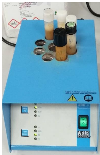
Figure 60: Cell Test Digester. Source: Own
