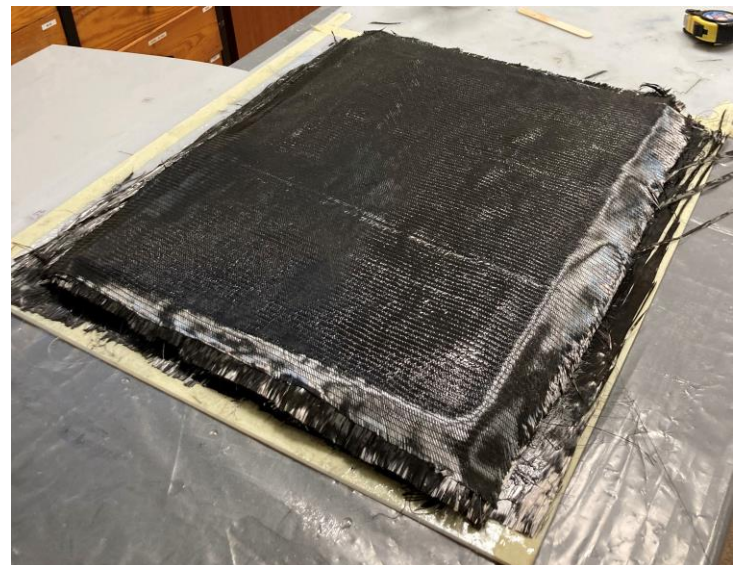
Figure 58: Hand lay-up process completed
