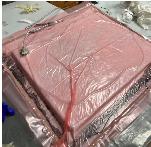
Figure 59: Vacuum bag on the sandwich
