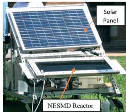
This NESMD solution is still under development since the membrane is manufactured in the laboratory as it is not available on the market. Unlike other distillation systems, this one has a solar panel that provides the extra energy needed to reach the boiling point of the water. Finally, it should be noted that this system is capable of producing a flow rate of 0.75 l/(m<sup>2</sup>\*h) which makes it less productive than other standard solutions on the market.
