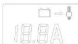
Discharge current from battery to load
