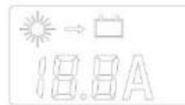
Charging current from solar panel to battery
