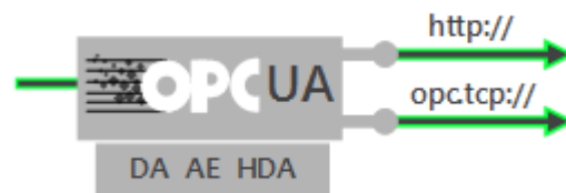
Figure 20. OPC UA transport mechanisms (Inmation, 2021).
