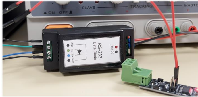
Figure 81. Data diode and USB to RS-232 converter.
