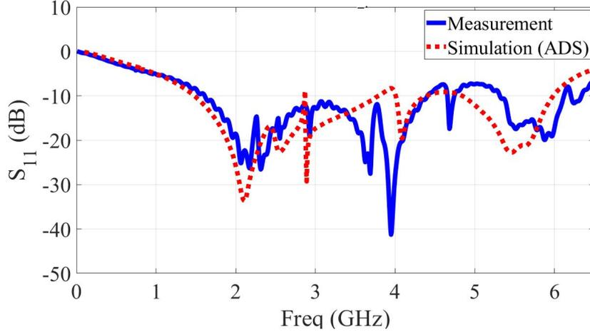
Figure 5.6: Frequency response (scattering parameters) of the SDD.
