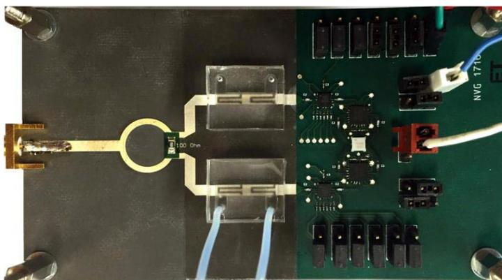
Figure 2.20: Improved sensitivity in a wideband operation(4.2 –8 GHz) using the nonlinear dispersion characteristic of metamaterial TL [94]
