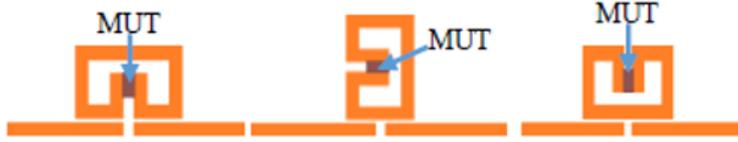
Figure 2.6: Half-wavelength resonator coupled to a microstrip TL in different orientations [51]
