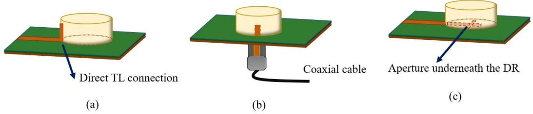
Figure 3.1: Different common feeding techniques applied to DR: (a) direct feeding using microstrip TL, (b) probe feeding, inserted inside the DR, (c) aperture feeding method.
