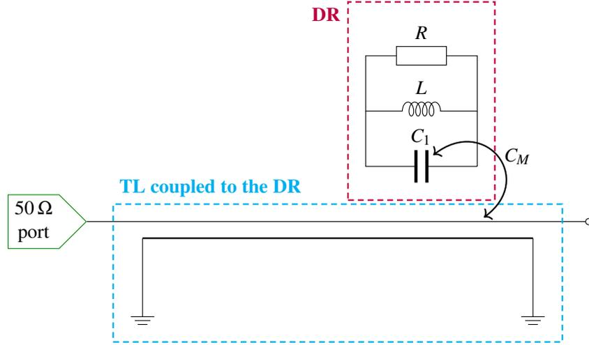
Figure 3.3: Circuit model of the DR coupled to the microstrip transmission line. The cylindrical cavity resonator is modeled as a parallel  $RLC$  circuit where  $R$ ,  $L$ , and  $C_1$  are defined as the parallel resistance, inductance and capacitance of the DR. The  $C_m$  capacitor is influenced by loading lossy liquids in the tank which is located on the sensitive area of the DR and accordingly the equivalent capacitance value ( $C_1 + C_m$ ) is changed.
