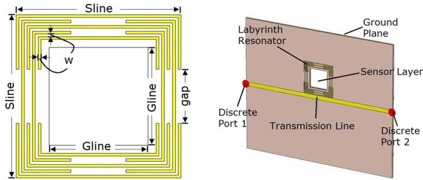
Figure 2.5: Labyrinth resonator in a broadside coupling to the microstrip TL [49]
