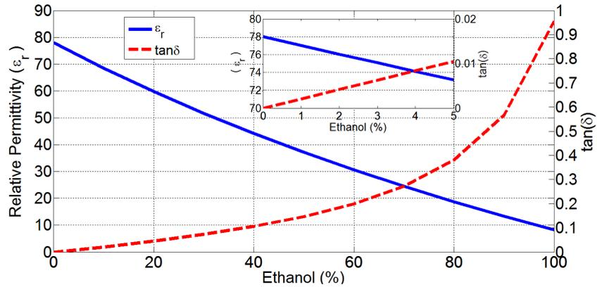
Figure B.1: Dielectric properties of the ethanol-water solution at 2.45 GHz.
