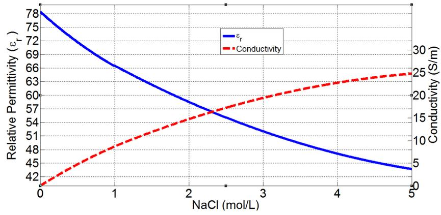
Figure B.3: Dielectric properties of the NaCl-water solution at 2.45 GHz.
