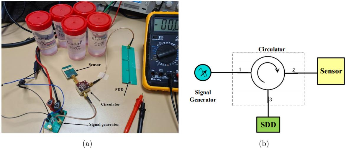
Figure 5.7: (a) Complete experimental setup including the VCO, SDD and sensor part attached to a circulator and (b) its block diagram.
