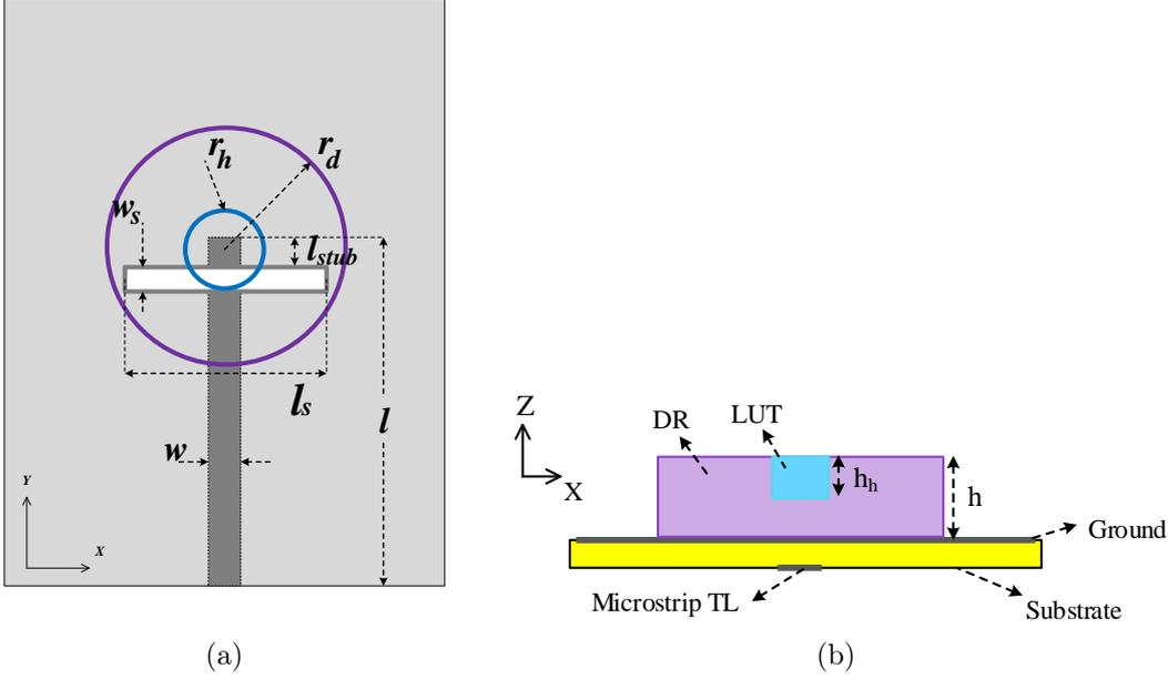
Figure 3.2: DR Sensor (a) Front view, (b) Side view, with generic dimensions. The prototype's dimensions are reported in Table 4.2.
