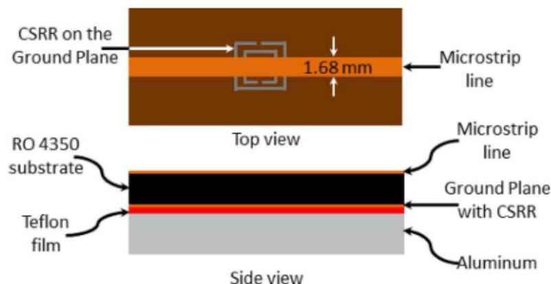
Figure 2.3: CSRR resonator etched on the ground plane of a microstrip TL [40]
