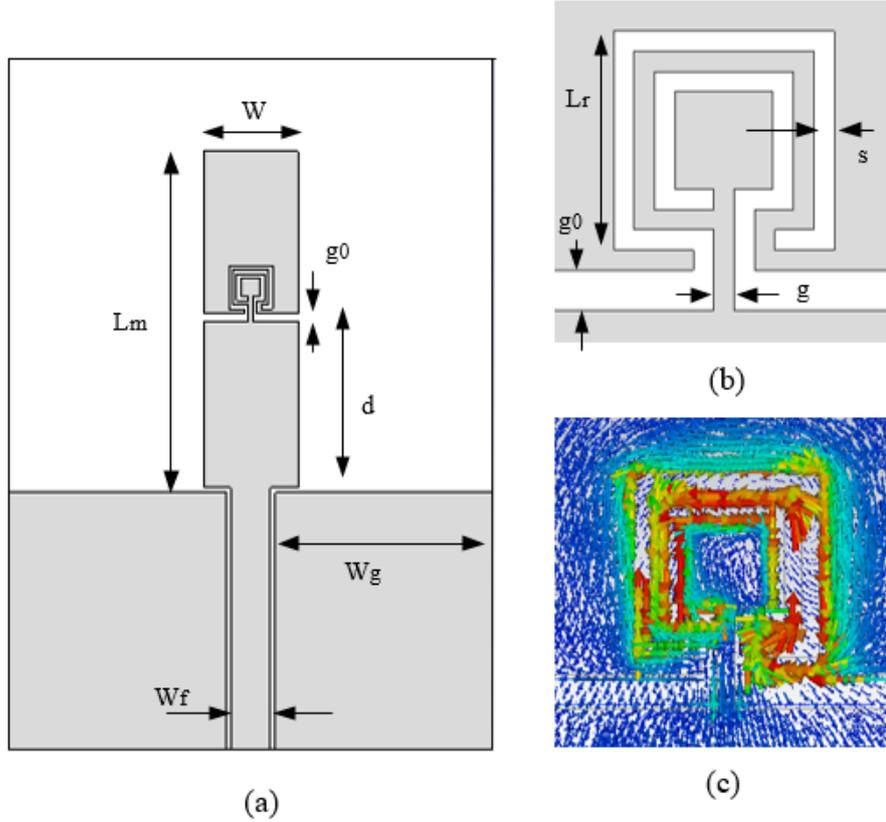
Figure 5.1: (a) Schematic layout of sensor, (b) OCSR loaded as the sensitive area and (c) current distribution at the resonant frequency of OCSR (i.e., at 4.74 GHz). The dimensions in mm are:  $W = 5.85$ ,  $L_m = 21$ ,  $W_g = 13.5$ ,  $g_0 = 0.5$ ,  $d = 12.5$ ,  $W_f = 2.44$ ,  $g = 0.25$ ,  $s = 0.25$ ,  $L_r = 2.3$ .
