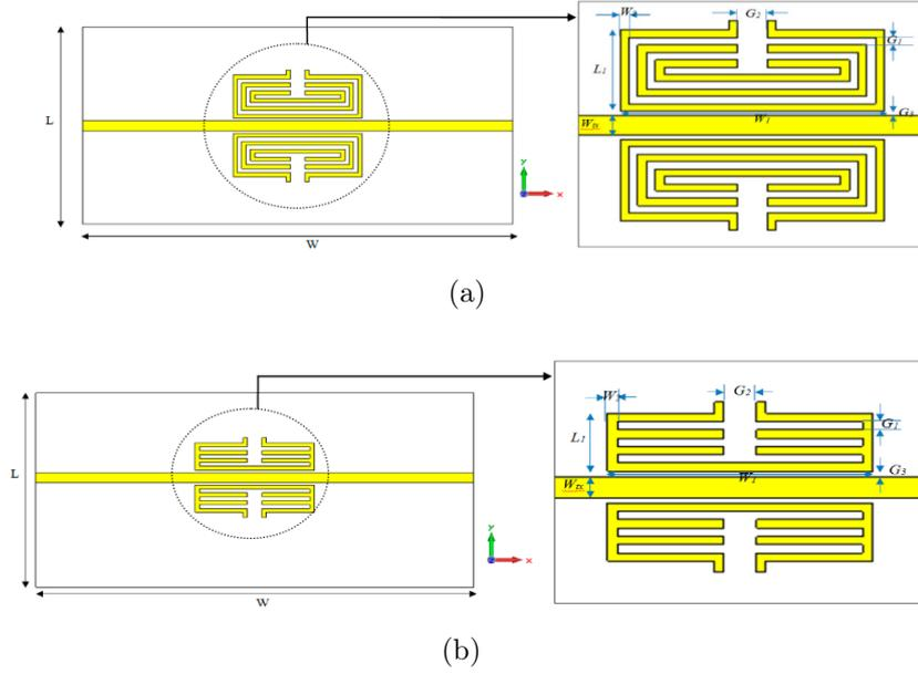
Figure 2.8: Schematic view of the (a) aligned gap and (b) centered gap [53]
