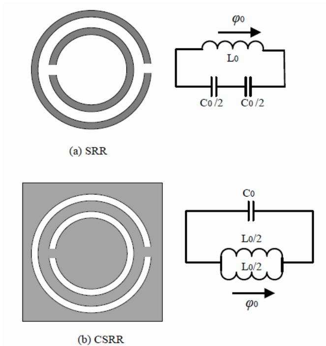
Figure 1.1: Topology of circuit models of (a) Split Ring Resonator (SRR) and (b) complementary SRR and equivalent [16]
