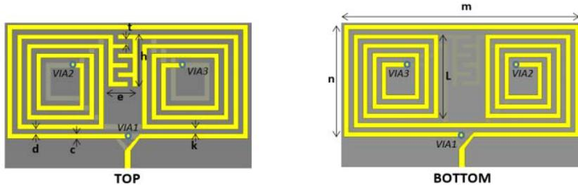
Figure 2.7: Attempts made to increase the sensitivity, double-sided spiral-ring resonator [52].
