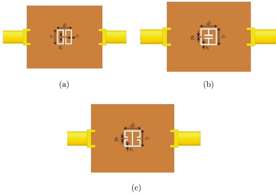
Figure 2.21: Differential sensors based on (a) CS-SRR, (b) CAS-SRR, (c) CBS-SRR etched on the ground plane of microstrip TL [96]
