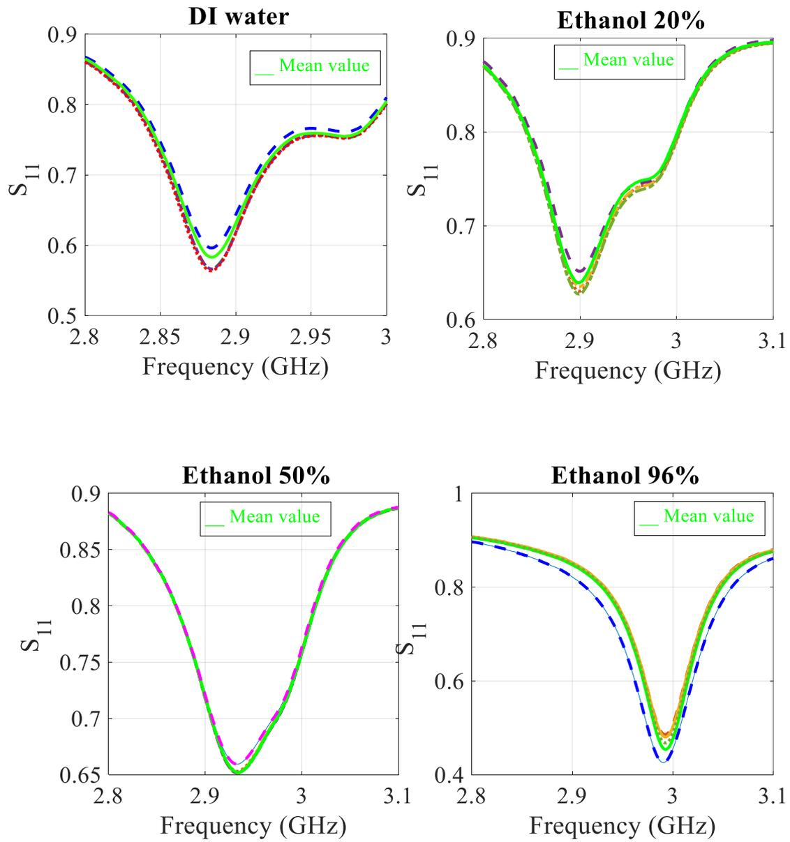
Figure 4.10: Measured scattering parameters of the un-shielded DR sensor for ethanol concentrations, each experiment has been repeated 5 times and the green line shows the mean value
