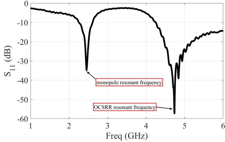
Figure 5.2: Measured reflection coefficient of the sensor part
