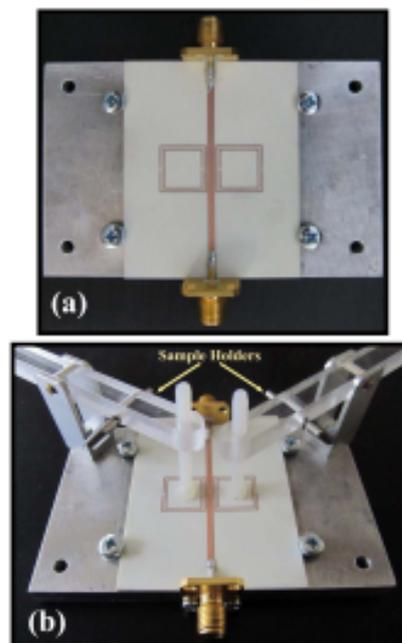
Figure 2.18: Microstrip TL coupled to identical SRRs with two non-identical samples creating two split notches as a differential sensor [88]
