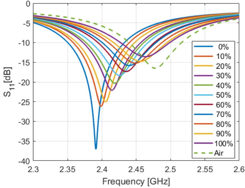
Figure 4.2:  $S_{11}$  simulated sensor response to different ethanol-water concentrations. Lines indicate the percentage of ethanol in water.
