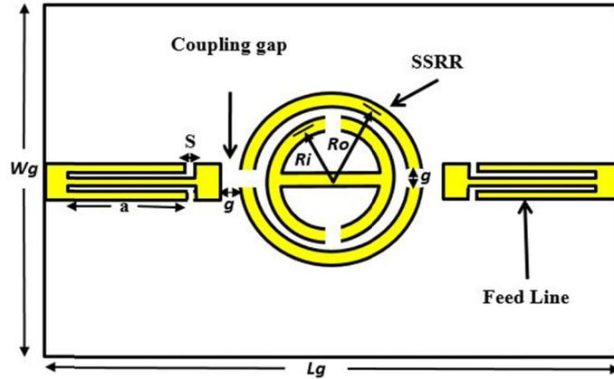
Figure 2.4: Symmetrical Split Ring Resonator (SSRR) is applied to spur-line feed lines [48]
