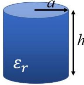
Figure 1.3: Schematic of the dielectric resonator made up of the ceramic material with permittivity  $\epsilon_r$ .
