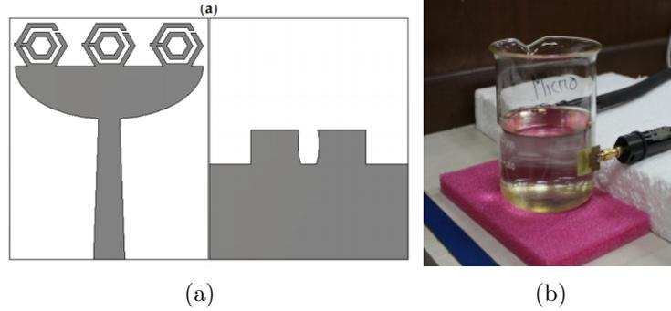
Figure 2.9: UWB monopole antenna loaded by three metamaterial unit-cells [58]
