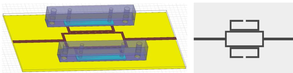
Figure 2.19: Differential sensor using splitter/combiner and microfluidic channels placed on top of the gap region of the SRRs [89]
