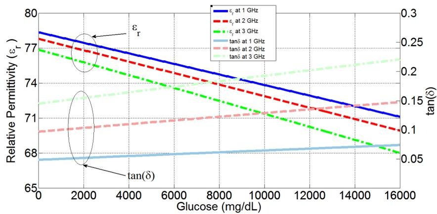
Figure B.2: Dielectric properties of the Glucose-water solution at 2.45 GHz.
