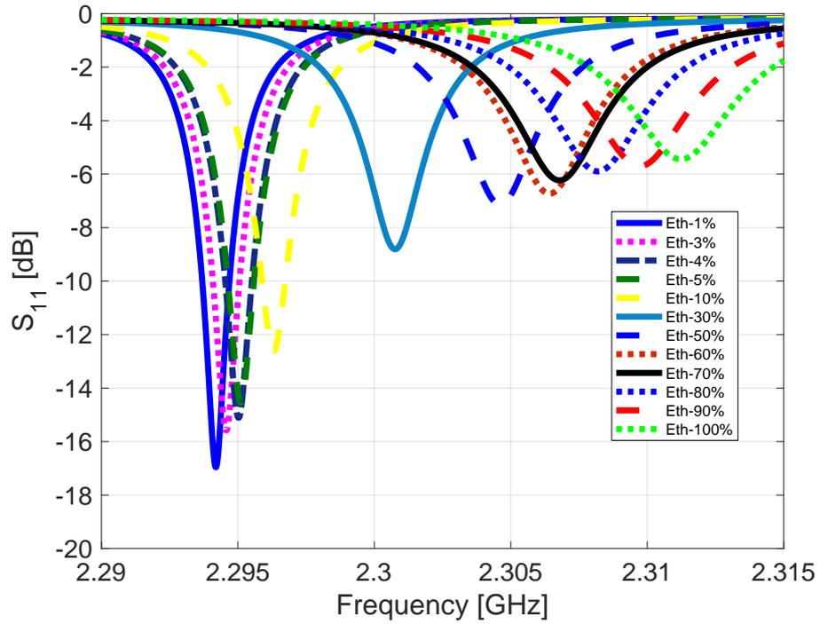
Figure 4.8: The frequency shift corresponding to the CST simulation of the DRS sensor for different ethanol concentrations
