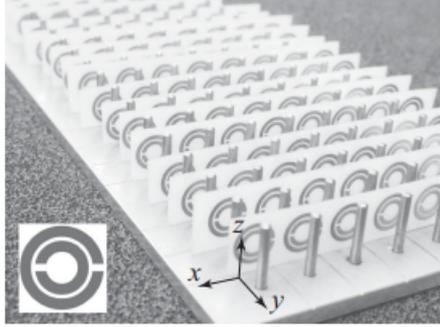
Figure 1.2: First experimental LH setup, structured by thin wires and SRR array to create a simultaneous negative permeability and negative permittivity [18].
