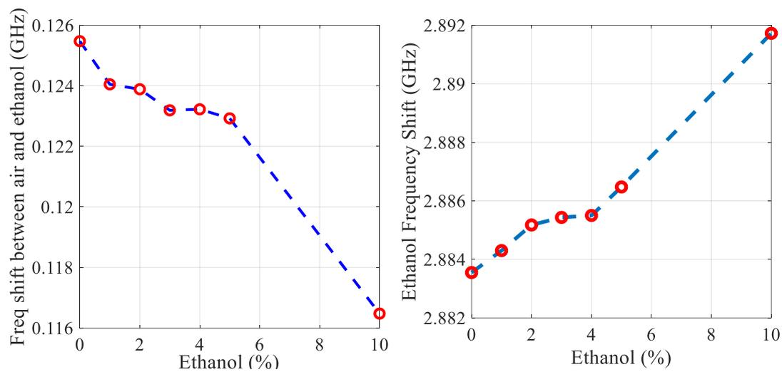
Figure 4.11: Sensor response for different ethanol concentrations.
