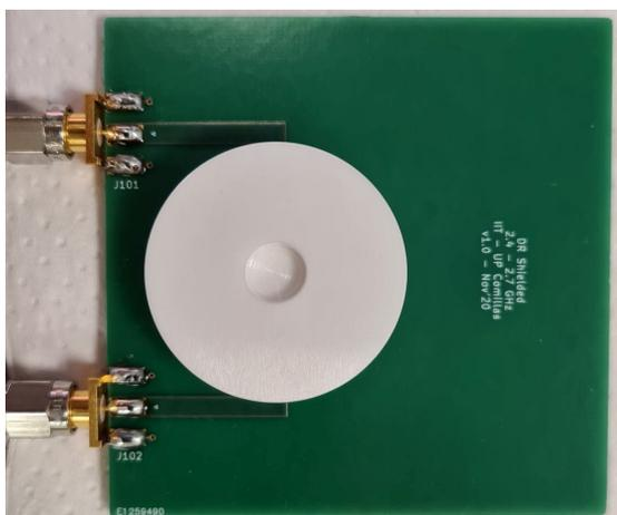
Figure 4.6: DR sensor in coupled-line feeding configuration without metal shield.
