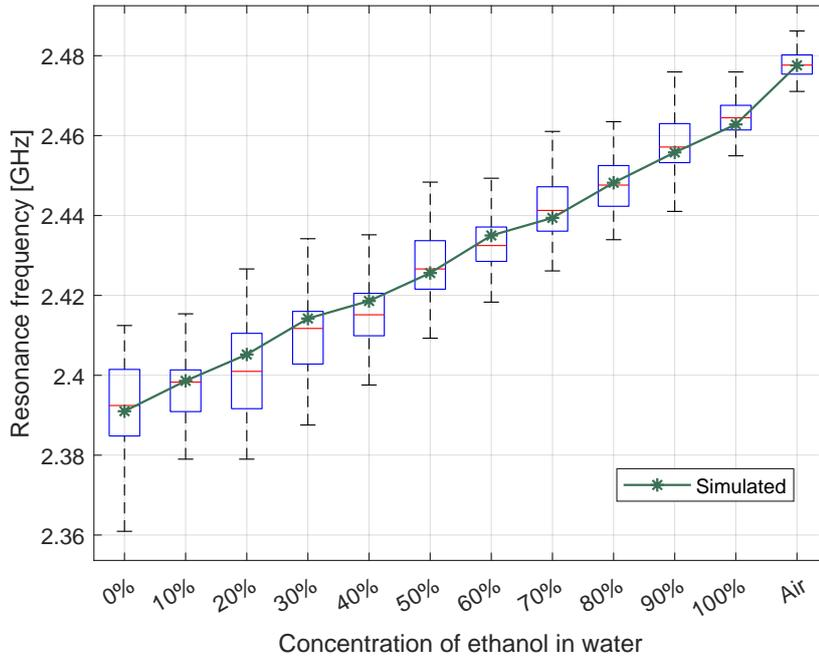
Figure 4.5: Statistics of the resonance frequency as a function of the ethanol concentration. Boxplots are for measured data (mean value and standard variation over 61 experiments per concentration) while the line is for the simulated sensor.
