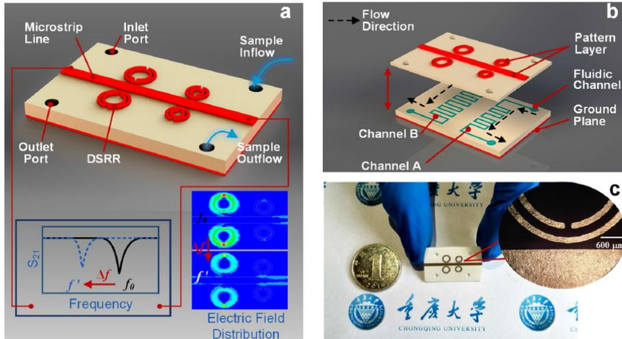
Figure 2.15: Multiband sensor including a meander microfluidic channel implemented beneath the resonators in order to increase the sensitivity [76].
