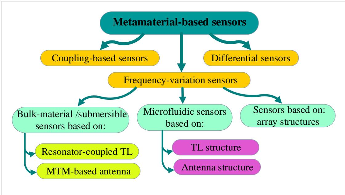
Figure 2.1: Classification chart of metamaterial sensors
