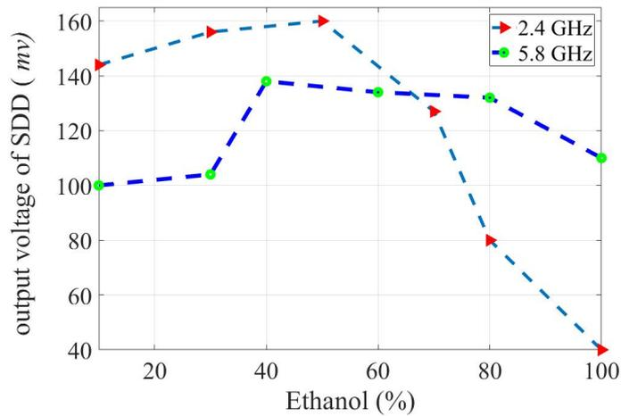
Figure 5.8: Measured SDD output voltage for different ethanol percentages at two different frequencies.
