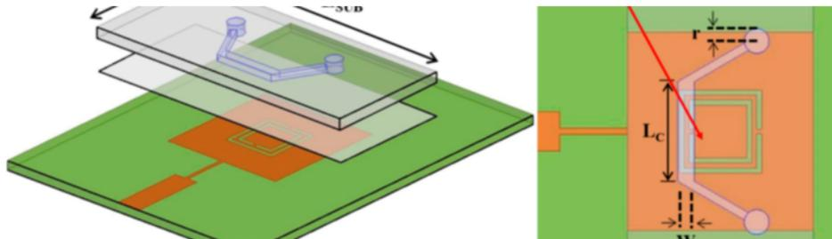
Figure 2.16: Monopole antenna applied as a microfluidic MTM sensor [77]
