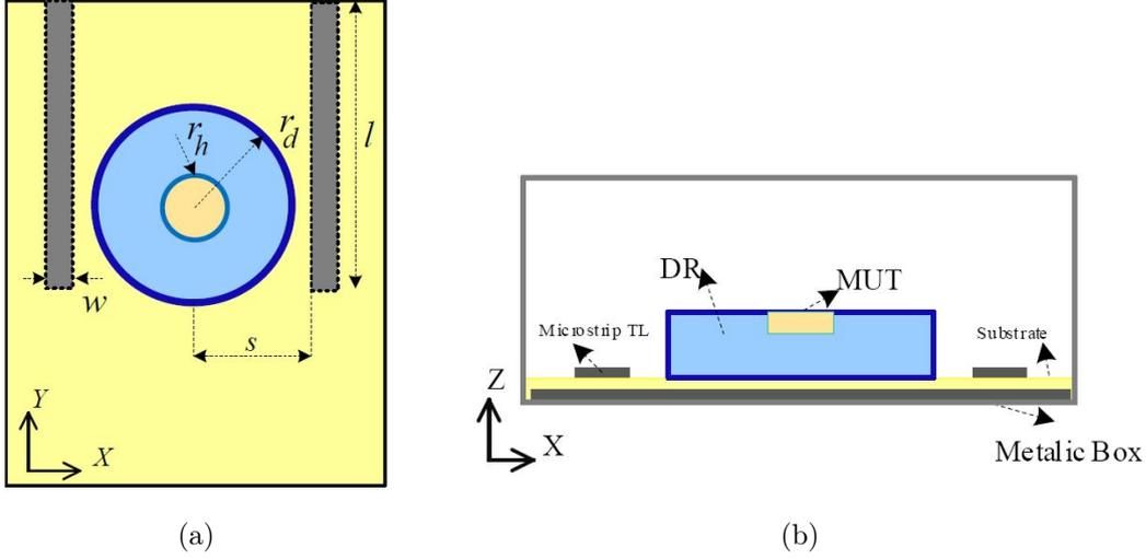
Figure 3.4: Shielded DR sensor fed by a parallel microstrip transmission line (a) Front view and (b) Side view, the dimensions are  $l = 30$  mm,  $s = 17.4$  mm,  $w = 2.95$  mm,  $r_d = 17$  mm,  $r_h = 4$  mm. The same DR in DRA sensor is used.
