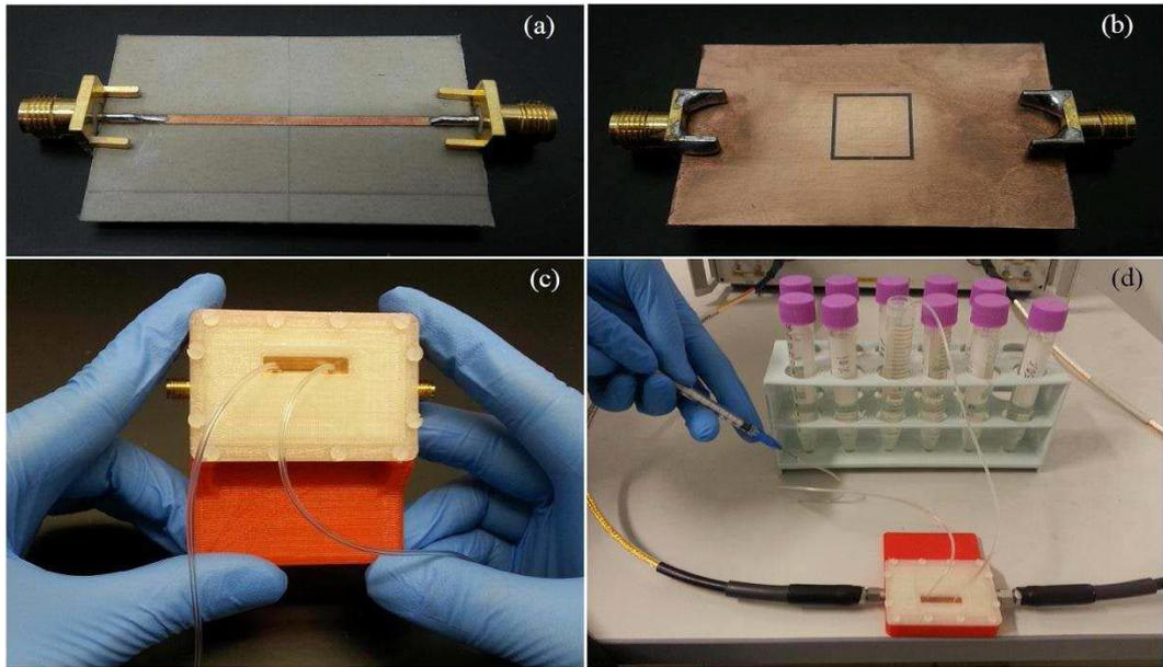
Figure 2.14: CSRR coupled to TL implemented by the microfluidic channel [72]
