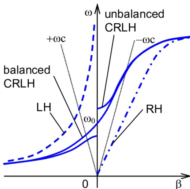
Figure 2.12: Dispersion diagram for left- and right-handed transmission lines. Dashed-dotted: conventional (right-handed) transmission line; dashed: idealized left-handed TLM; solid: composite right/left-handed TLM for the balanced case (continuous line) and unbalanced (discontinuity at  $\beta=0$ ) [70].
