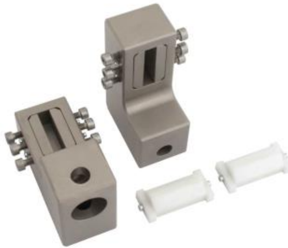
Illustration I. Design reference for Arcan testing fixture (Universal Grip Co.)
