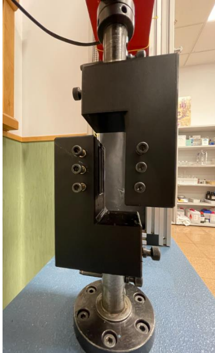
Illustration VI. Assembly on testing machine of Arcan testing fixture
