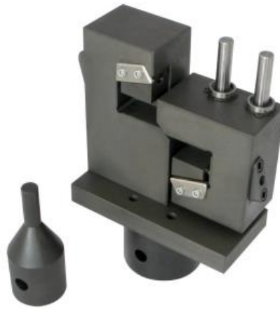
Illustration III. Design reference for Iosipescu testing fixture (Universal Grip Co.)
