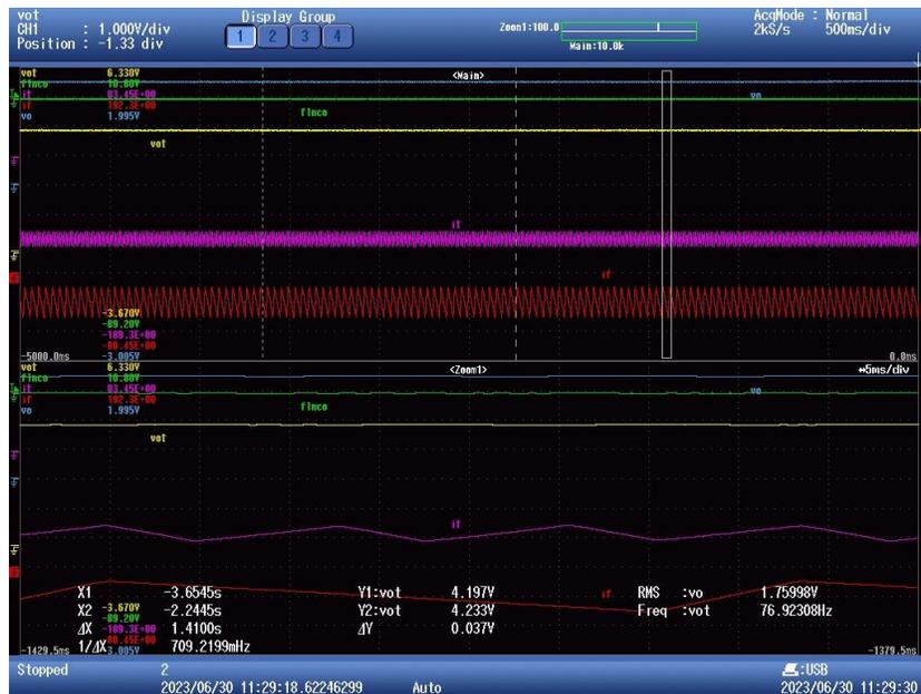
Figure 3. Example of oscilloscope reading. (Yellow - Vout. Red- Current of one of the phases. Purple- sum of current of all phases).
