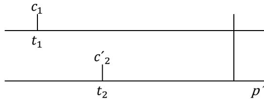
$$c_1 (1 + i)^{(p'-t_1)} = c'_2 (1 + i)^{(p'-t_2)}$$
