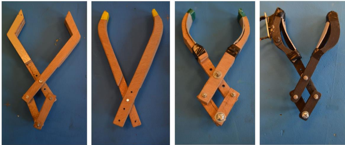
Figure 15. The four versions of the gripper fingers (in order of creation, from left to right).
