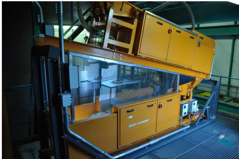
Figure 7.6: Two in series inclined ECS configuration [ZAR11]
