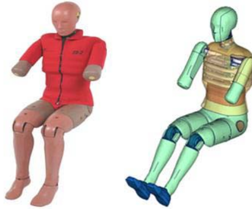
Figure 2.8: EuroSID-2 Dummy. Real model (left) and CAE model (right).
